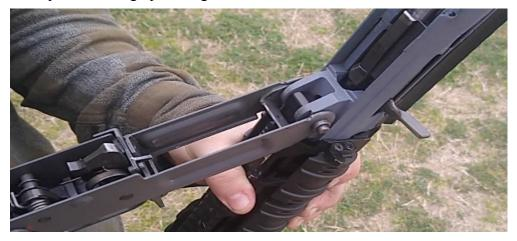
3. insert the gun adapter (V shaped item) on top of front of the magazine well.
